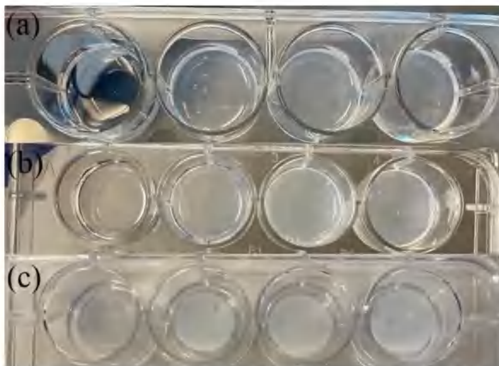
Figure 1. Macroscopic images of at the different stages of the synthetic process: (a) acidic mixture (pH 3.6) left at 37 °C overnight, (b) after washing with citrate solution (pH 7.2) to neutral pH and (c) after incubation with thrombin in citrate at 37 °C overnight. Final concentrations: fibrinogen = 20 mg.mL -1 , collagen (from left to right) = 0, 2.5, 5, 10 mg.mL -1 .
