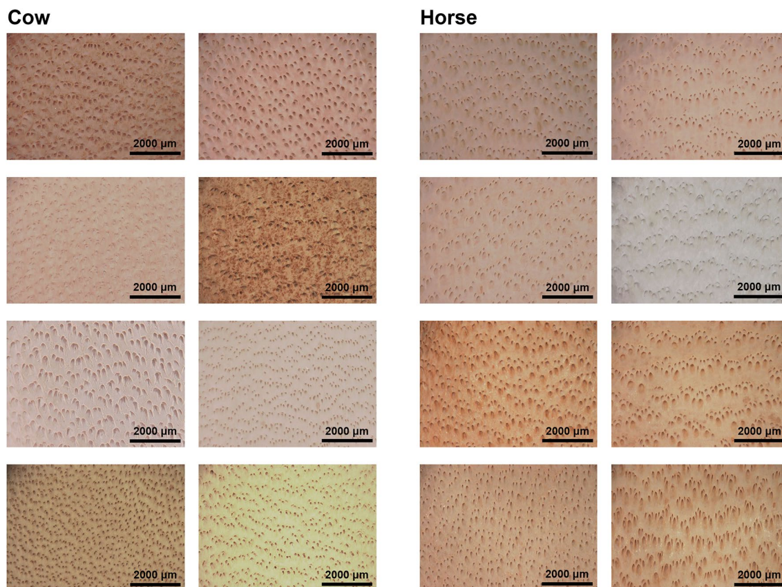
Fig. 1 Digital microscope images of cowhides and horsehides
