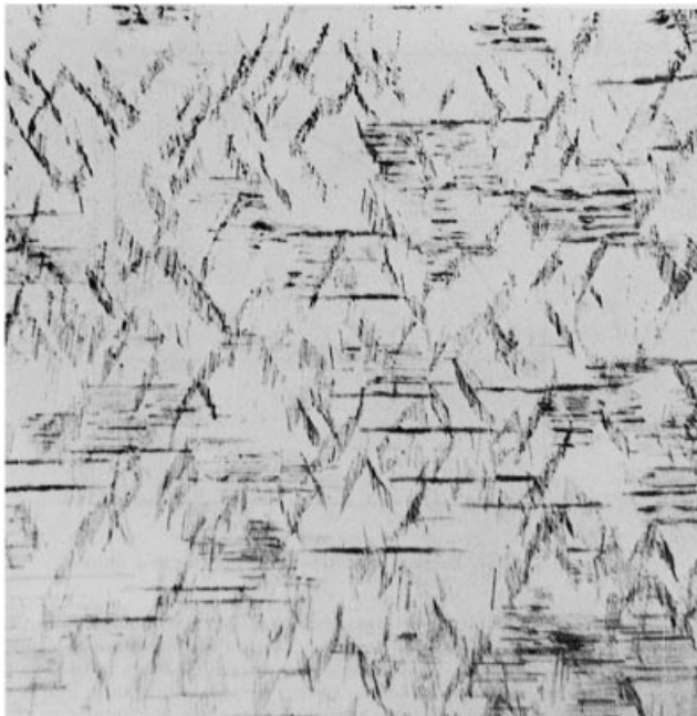
Fig. 9. Transmission electron micrograph at 40,000 magnification showing S'-phase precipitates in Al-Cu-Mg alloy sheet aged 12 h at 100°C.
