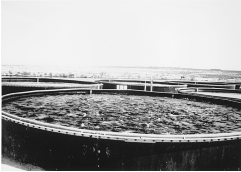
Fig. 4. Circular tanks are a raceway option. They can be placed outdoors or used in conjunction with indoor water systems. Circular tanks are commonly used in recirculating systems.
