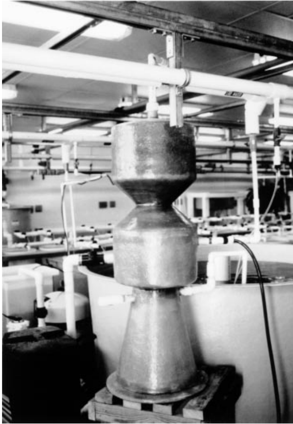
Fig. 7. A bead filter, one of many types of biological filters, shown in association with a laboratory-scale recirculating water system. Small plastic beads inside the fiberglass chamber provide surface area for colonization by bacteria that convert ammonia to nitrate.
