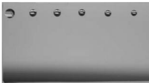
Fig. 11. Digital optical photographs of a PS/PVME T - \phi library after 91 min of annealing, showing the LCST cloud point curve visible to the unaided eye. White circles are conventional light-scattering cloud points measured on separate uniform samples. Picture adapted from cover of Macromolecules , 2001.
