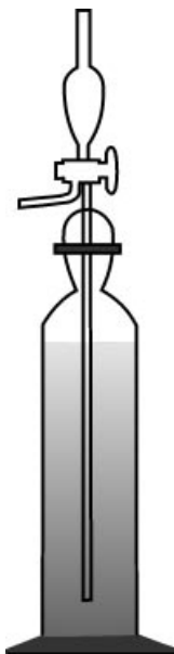
Fig. 11. In the Andreason sedimentation pipette, the cylinder is filled with homogeneous dispersion. The concentration at the sampling depth is measured as a function of time (14).
