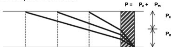
(c) Pressure profiles for a constant pressure filtration of an incompressible filter cake and nonnegligible constant medium resistance. The total pressure drop equals the sum of the pressure drops over the filter cake and the filter medium. For a constant pressure filtration the pressure drop over the medium decreases as the cake depth increases and cake contributes to more of the total pressure drop.
