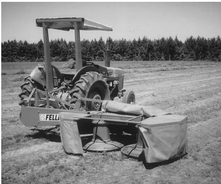
Fig. 6. Drum mower successfully used to harvest flax fibers for nontraditional applications. With mowing, fiber alignment is not maintained and fiber yield is less due to the remaining stubble. Costs may be less due to use of general-purpose farm equipment.
