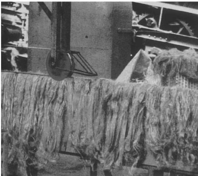
Fig. 14. Flax stems that have been retted and scutched for traditional linen production are long, aligned, and clean fiber bundles. These fibers, which will be further cleaned by hackling, are eventually wet spun for high value, 100% linen materials.
