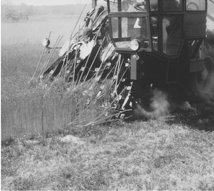
Fig. 5. Pulling of flax using specialized equipment produced in Europe. Stems with roots attached are pulled to maintain a high yield of long, strong fiber bundles for traditional linen production.
