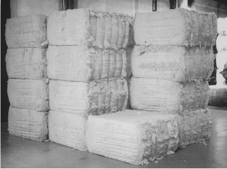
Fig. 16. Bales of cottonized flax from total fiber processing systems. Flax cleaned in this way can be non-uniform in length or further processed or cut for a more uniform length. Cottonized flax is cleaned and refined for blending with cotton and other fibers for short staple spinning systems.
