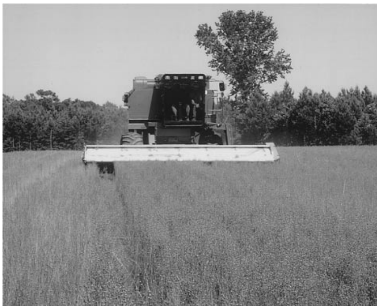
Fig. 7. A stripper-header used to harvest linseed, leaving the stems upright for subsequent harvesting for fiber.
