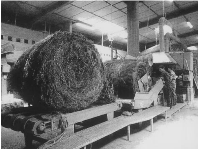
Fig. 13. Round bales of dew-retted flax entering a bale opener, which is the beginning of mechanical processing where stems will be broken and fibers cleaned of contaminants.
