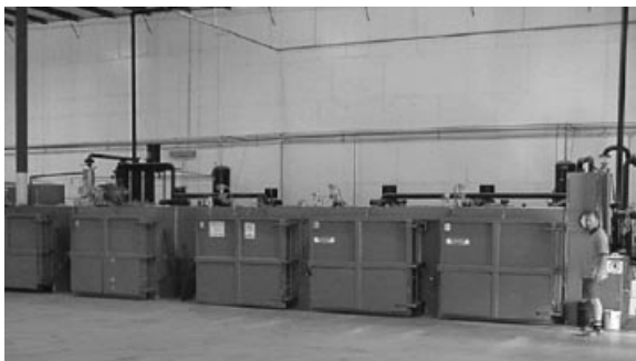
Fig. 5. Parts are loaded into large reactor chambers, air is removed via a vacuum pump, and a gas blend containing fluorine is added. Temperature within the chamber can be controlled through jacketing on the reactors. After a predetermined reaction time has elapsed, the chamber is evacuated via a vacuum pump, with effluent gas being neutralized in a caustic scrubber. The chamber is refilled with air, opened, and the surface treated parts are removed.
