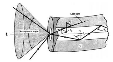
Fig. 12. Light guiding in a clad fiber (99).
