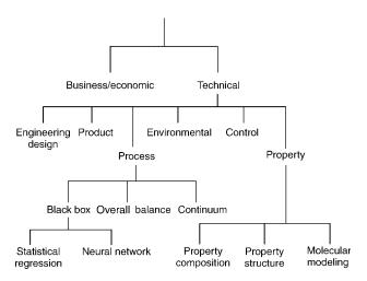
Fig. 19. Classification of mathematical models used in the glass industry (201).
