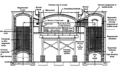
**Fig. 18.** Cross-section of typical regenerative sideport glass-melting tank. Gas and heated air enter at inlet A and the mix goes then to the burner blocks. The flame goes into the furnace across the top of the glass batch (B) while exhaust gases are withdrawn through the regenerator C. After a 15–20-min cycle, the process is reversed (from C to A) which allows efficient use of energy (159).
