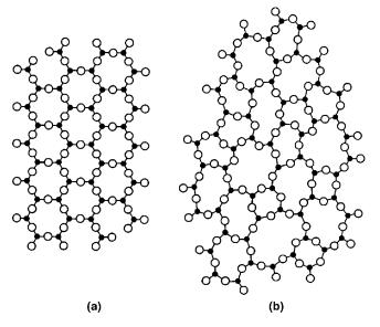
**Fig. 4.** Schematic two-dimensional (2D) representation of the silica random network built by  $SiO_4$  tetrahedra: (a) crystalline structure (or long-range order), (b) random network (7).
