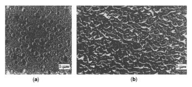
**Fig. 11.** Microstructural morphology of immiscibility in glasses: (**a**) sodium-borosilicate glass showing a nucleated type of phase separation, and (**b**) sodium-borosilicate glass composition from center of immiscibility region (spinodal decomposition) (90).
