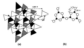
Fig. 7. (a) Structure of crystalline  $B_2O_3$  formed by  $BO_3$  triangles and (b) boroxol unit (20).
