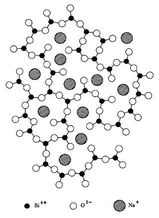
Fig. 5. Schematic 2D representation of the random network of alkali silicates (11).
