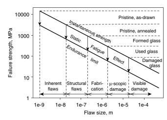
**Fig. 15.** Effects of crack size (including those generated from typical processing and handling) and fatigue processes on strength in silica glass (150).
