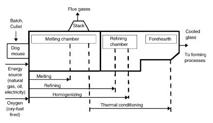
Fig. 17. Melting and refining processes (158).
