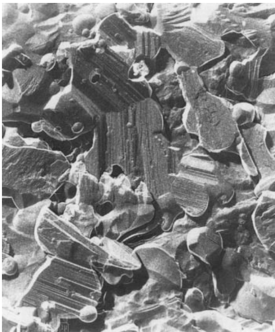
Fig. 2. Replica electron micrograph of the fracture surface of enstatite- \beta -spodumene-zirconia glass-ceramic, showing twinning in the enstatite grains (white bar = 1\mu\text{m} ).
