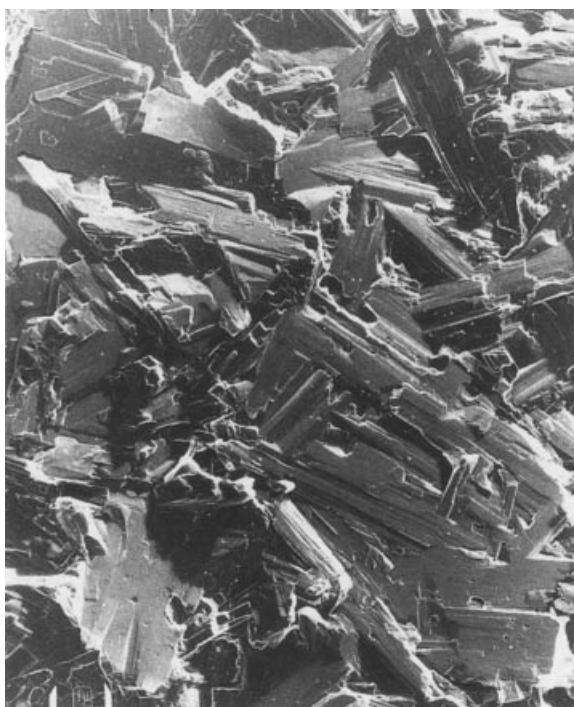
Fig. 4. Fracture surface (replica micrograph) of fluorcanasite glass-ceramic showing interlocking blade-shaped crystals and effects of cleavage splintering (white bar = 1 \mu\text{m} ).
