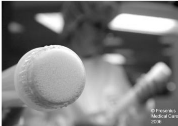
Fig. 5. Photograph of dialyzer without end cap at Fresenius plant in St. Wendel, Germany. Copyright Fresenius Medical Care (2006). Reproduced with permission.
