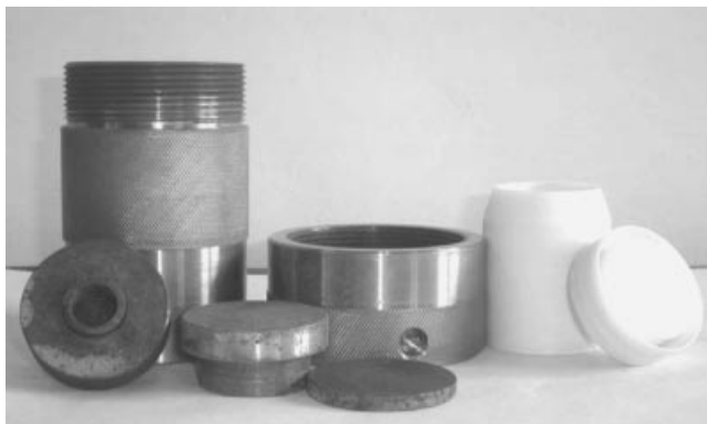
Fig. 5. General purpose autoclave popularly used for hydrothermal treatment and hydrothermal synthesis.
