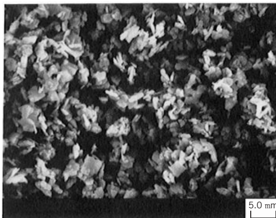
Fig. 3. Aluminum oxide–hydroxide: hydrothermally prepared boehmite, \times 2,000 . Courtesy of Aluminum Company of America.
