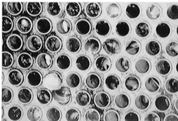
Fig. 14. Surface condenser infested with adult Asiatic clams.
