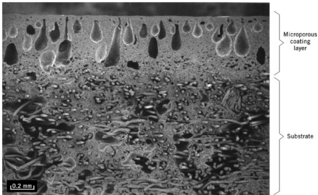
Fig. 6. Cross-sectional view of Clarino.
