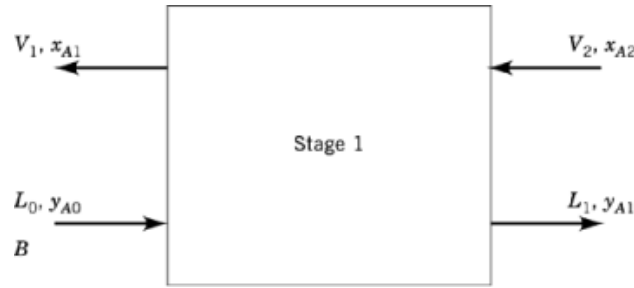
Fig. 1. Flow diagram for single-stage leaching.
