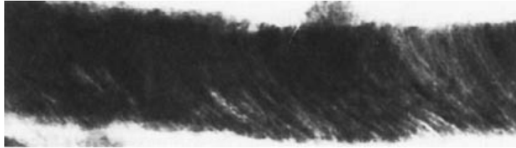
Fig. 21. Transmission electron micrograph (tem) made from a cross-section of a metal-evaporated tape medium with the typical banana-like shape of columns. The layer thickness is \sim 120 nm.
