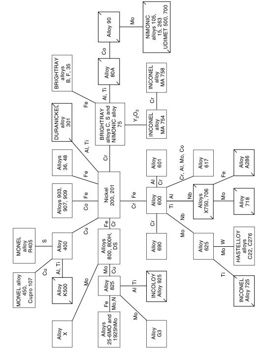
**Fig. 1.** Development of wrought nickel alloys (see Tables 5 and 6), where ( $\Lambda$ ) represent solid solution material and ( $\Box$ ) represent precipitation-hardenable material. Alloys 25-6MO and 1925hMo are superaustenitic stainless steels.
