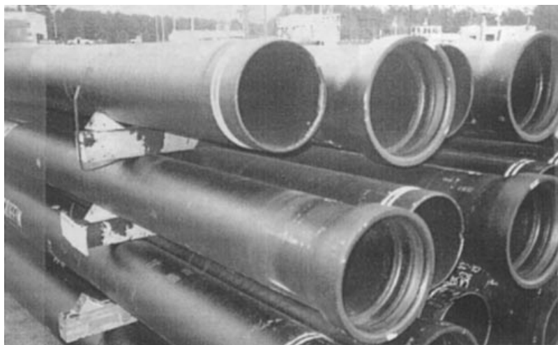
Fig. 5. Ductile iron pipe common in waterworks.
