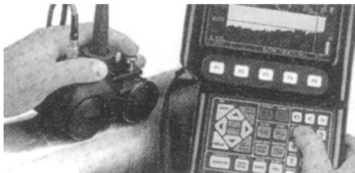
Fig. 14. Ultrasonic testing of wall thickness.
