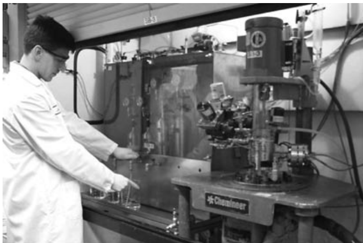
Fig. 5. Laboratory equipment for emulsion polymerization at high pressures. (Photograph courtesy of BASF Corporation.)
