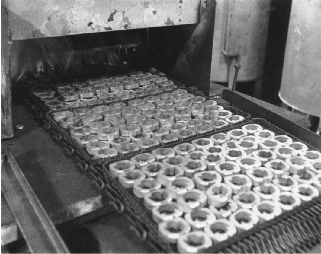
Fig. 3. Sintering of the green compact in a controlled atmosphere furnace.
