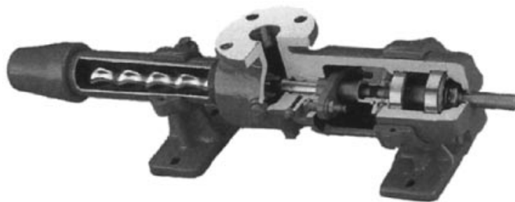
Fig. 11. Radial and lateral clearances of gear pumps. A stainless steel pump employs stainless drive gear driving the Teflon idler. Shafts are supported by the carbon bushings and carbon wear plates. Courtesy of Liquiflo Equipment, division of Picut Industries.
