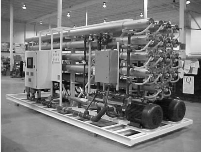
Fig. 2. A photo of a typical full-scale RO membrane module (spiral-wound) system capable of producing 500,000 gal/day (1892.7 m 3 /day). Note: Each tube (pressure vessel) contains six spiral wound modules. (Courtesy of GE Osmonics.)
