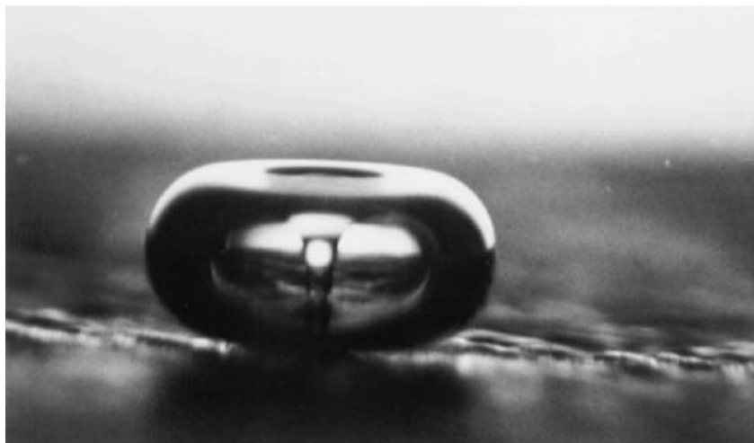
Fig. 3. Liquid jet produced during collapse of a cavitation bubble near a solid surface. The width of the bubble is about 1 mm. (Reproduced with permission (8).)
