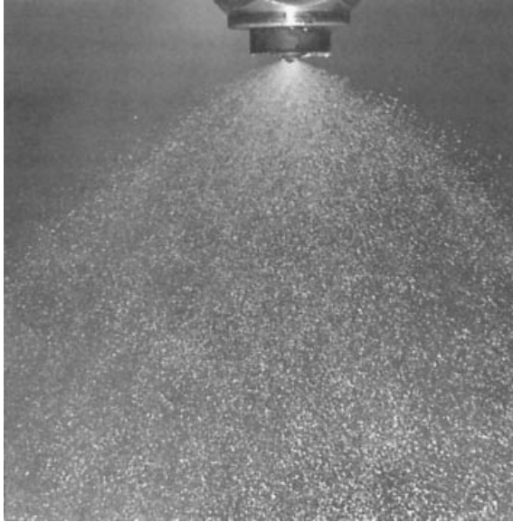
Fig. 3. Supercritical fluid atomization process.
