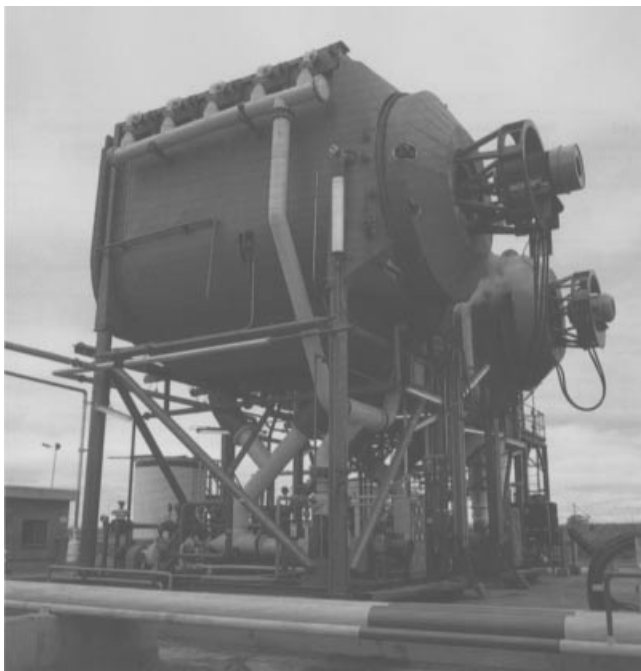
Fig. 10. A two-stage 700-m 3 /d VC brine concentration plant. (Courtesy of I.D.E. Technologies Ltd.)
