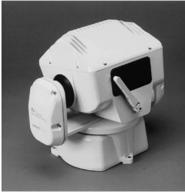
Fig. 5. The Night Sight commercial thermograph made for all-weather operation uses the uncooled pyroelectric focal plane.(Courtesy of Texas Instruments Inc.)
