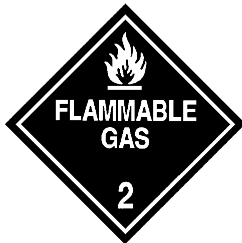
Fig. 2. Placard signifying the presence of a flammable gas. The numeral in the lower corner represents the primary hazard class of the material in the transport vehicle (62).
