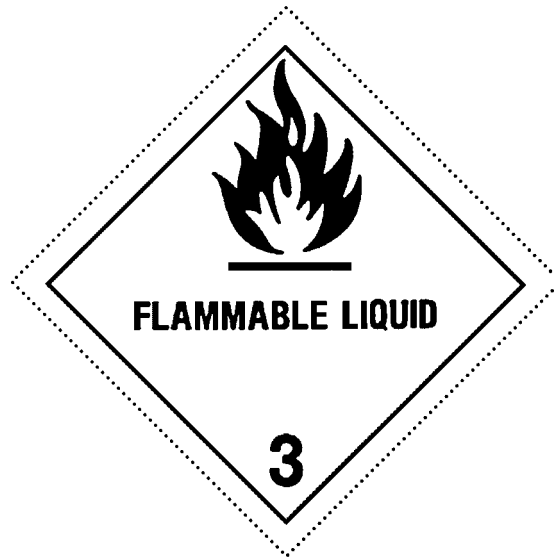
Fig. 1. Label signifying the presence of a flammable liquid. The numeral in the lower corner represents the primary hazard class of the material in the labeled package.
