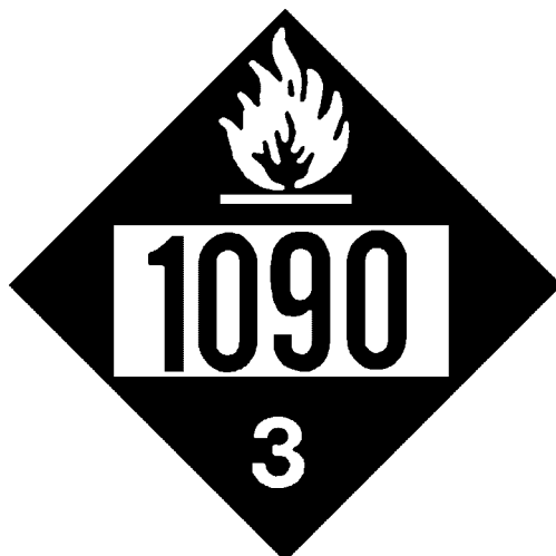
Fig. 3. Illustration of an identification number on a placard for acetone. The numeral in the lower corner represents the primary hazard class of the material (64).
