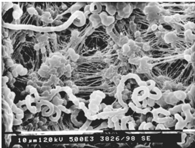
Fig. 19. Scanning electron microscopy (SEM) micrograph of the surface of a polyethylene particle formed on a \text{MgCl}_2 -supported catalyst.
